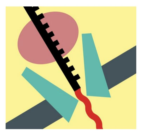
Conceptual rendering of the peptide reader, where a helicase (red) pulls up a DNA molecule (black) to which a peptide (red) is attached—yielding a slow translocation of the molecule through the nanopore (green) which allows to read off the ion current signals that characterize the amino acids of the peptide as they temporarily block the pore. Credit: Henry Brinkerhoff, Cees Dekker Lab, TU Delft
