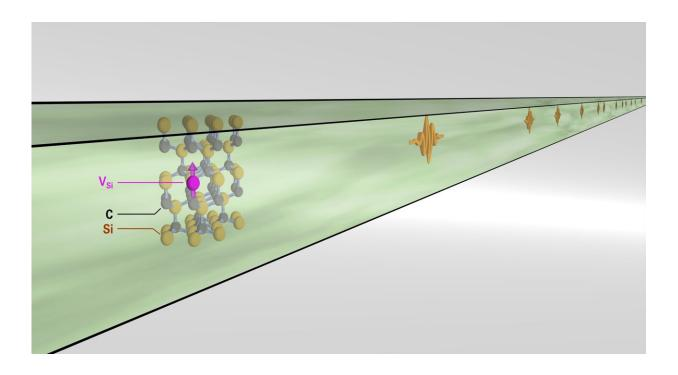
Visualization of a VSi center integrated into a nanophotonic SiC waveguide. Credit: University of Stuttgart / Physics 3
