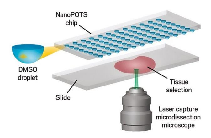
In this version of the nanoPOTS (nanodroplet processing in one pot for trace samples) sample-processing system adapted for imaging, cells isolated from tissue by laser capture microdissecton are captured by dimethyl sulfoxide (DMSO) nanodroplets on a glass slide. In a multistep process, the proteins are extracted from the cells and digested into peptides before analysis by liquid chromatography/mass spectrometry. Credit: American Chemical Society
