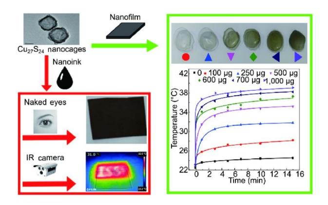
$Cu_{27}S_{24}$  nanocage was synthesized and evaluated by a combination of experimental measurement and theoretical calculation. And the developed  $Cu_{27}S_{24}$  "nanoink" and "nanofilm" showed high efficient photothermal performance. Credit: XI Min
