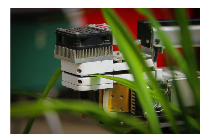
Infra-red gas analyzer and a rice leaf. The leaf is placed inside a cuvette in which conditions related to light intensity, CO2 concentration, relative humidity, and temperature can be controlled. Credit: International Rice Research Institute
