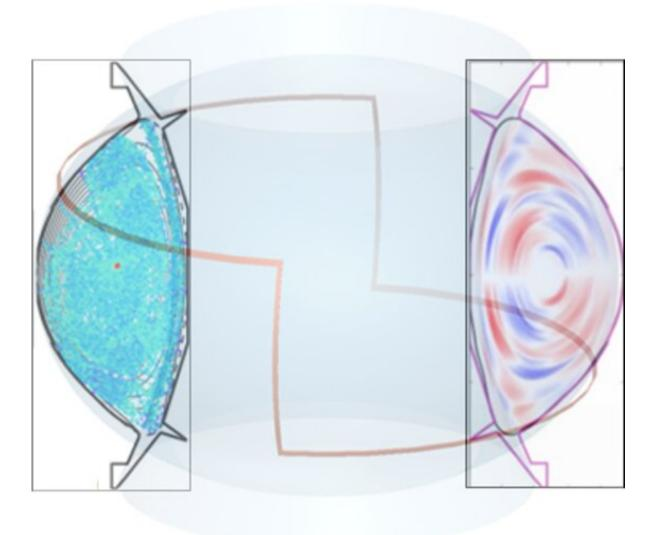
A composite image illustrating the operation of the runaway mitigation coil. The coil is shown as a heavy red line superimposed on the tokamak vacuum vessel (shown by the pale-blue shading). The insert on the right shows the perturbed
