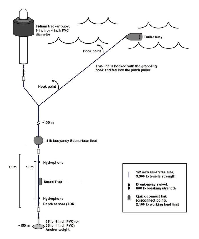
Schematic design of Pacific Island Fisheries Science Center—Drifting Acoustic Spar Buoy Recorder (PIFSC DASBR). Credit: DOI: 10.3389/fmars.2021.664292
