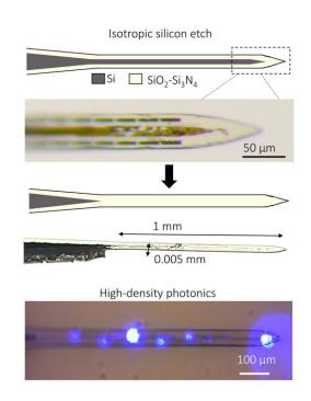
Thin and flexible glass-nitride probes fabricated from silicon substrates integrate electrode arrays and high-density photonics for neural readout and stimulation. Credit: Vittorino Lanzio
