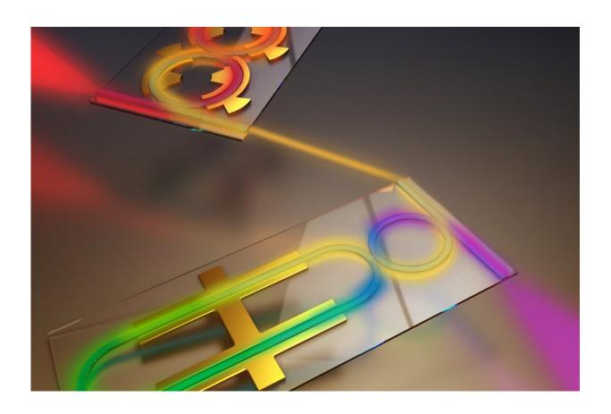
In the top device, two coupled resonators form a figure eight-like structure. Input light travels from the waveguide through the resonators, entering as one color and emerging as another. The bottom device uses three coupled resonators: a small ring resonator, a long oval resonator called a racetrack resonator, and a rectangular-shaped resonator. As light speeds around the racetrack resonator, it cascades into higher and higher frequencies, resulting in a shift as high as 120
