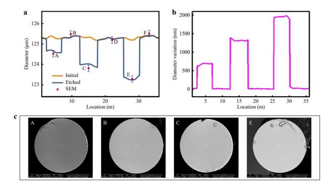
(a) Demodulated diameter distribution before and after etching and its comparison with the SEM results (A-F). (b) Diameter variations along the FUT. c Four representative images of the fiber cross-section at A, B, C, and E, captured by SEM. Credit: by Zijie Hua, Dexin Ba, Dengwang Zhou, Yijia Li, Yue Wang, Xiaoyi Bao and Yongkang Dong
