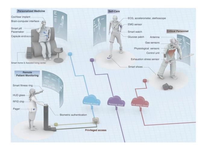
The internet of bodies (IoB) is a network of wearable, implantable, ingestible and injectable smart objects that allows for in-, on- and off-body communications. Credit: KAUST; Heno Hwang
