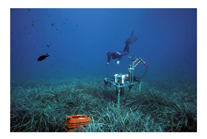
A researcher from the Max Planck Institute for Marine Microbiology taking samples in seagrass meadows in the Mediterranean Sea. The measuring device determines the oxygen content in the seabed. Credit: Hydra Marine Sciences GmbH
