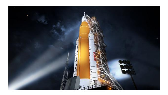
Nasa's new rocket, the Space Launch System (SLS), in its Block 1 crew vehicle configuration that will send astronauts to the Moon on the Artemis missions.
