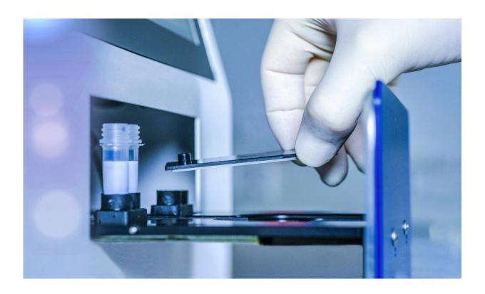
The compact device for detecting multidrug-resistant pathogens performs all stages of the reaction automatically and provides a result within one hour. Even one single DNA molecule is enough for detection. Credit: Fraunhofer IPM
