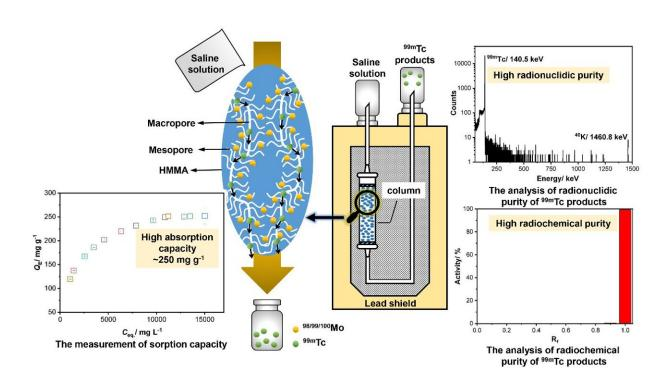
The investigation on preparation of LSA <sup>99</sup>Mo/<sup>99m</sup>Tc generator. Credit: WANG Jieru and QIN Zhi
