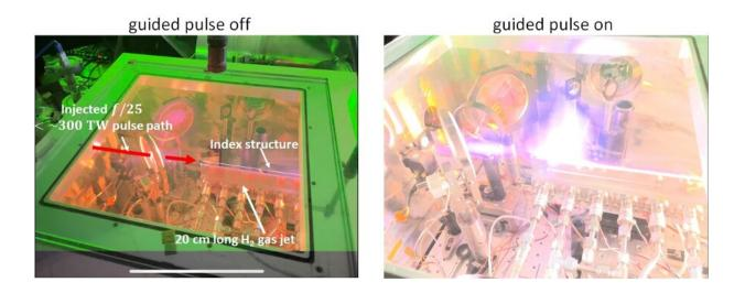
Photos of target chamber without and with injection and guiding of ultra-intense laser pulse into 20 cm long waveguide. Laser guiding leads to multi-GeV electron acceleration, with an intense burst of electrons emerging at the exit of the plasma waveguide (to the right). Credit: University of Maryland
