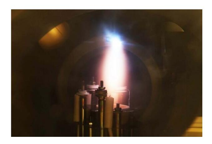
Plasma plume during an in situ PLD measurement. Credit: Vienna University of Technology
