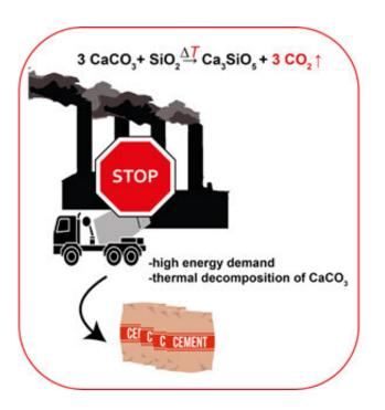
Conventional production of cement by burning lime and sand: during the reaction carbon dioxide is released. Credit: Marcel Maslyk
