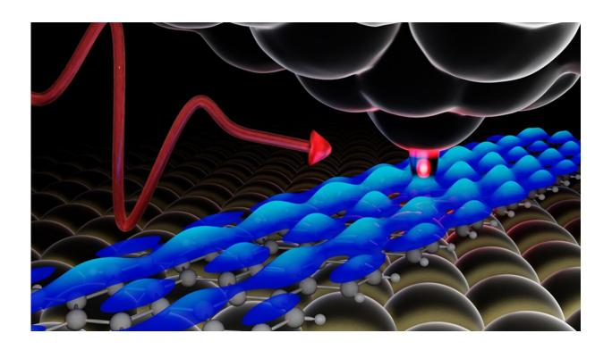
A schematic representing a microscopy measurement where a pulse of laser light (red curve) illuminates an atomically sharp needle (top) positioned above the sample surface. The graphene nanoribbon sits on top of a gold substrate. Experimental data is shown in blue, revealing the distribution of electrons above the nanoribbon. Credit: Spencer Ammerman
