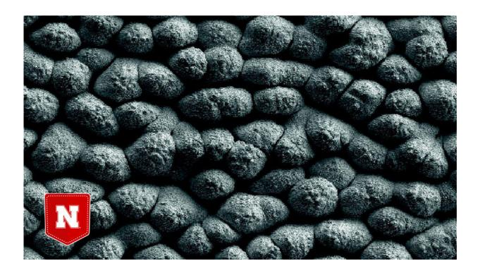
Microscopic mounds formed from a copper surface struck by 719 laser pulses and later treated with citric acid. Credit: *Thermal Science and Engineering Progress /* Elsevier
