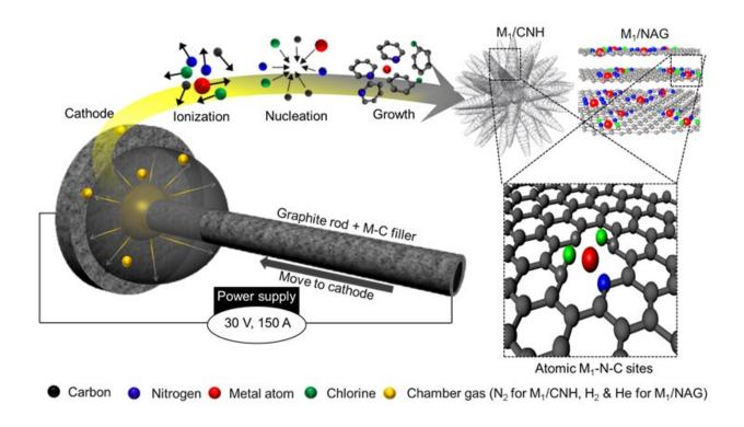
showing a single atomic catalyst synthesis reaction using artificial lightning. Credit: Korea Institute of Science and Technology (KIST)
