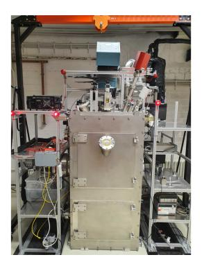
The new chamber, which will simulate space-like conditions and has 14 associated instruments to measure comet properties. Credit: Kreuzig et al.
