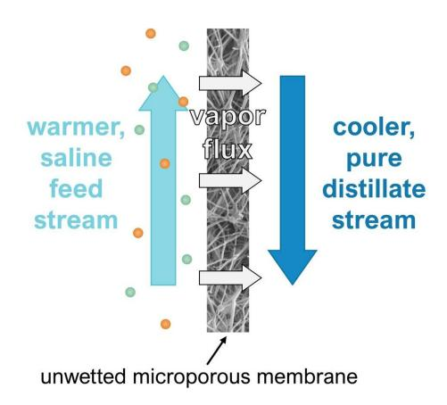
The warm high salinity water stream is on one side of the membrane and a cool pure water stream is on the other. the warmed water evaporates, leaving the salt behind and forming a vapor, which transforms to a distilled liquid form when meeting the cool water stream on the other side of the membrane. Credit: Allyson McGaughey.
