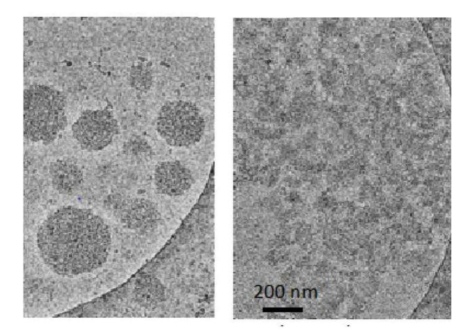
This Cryo-TEM image of native milk protein (casein) micelles in skim milk (left) and disordered open protein structures after high pressure jets at 400 megapascal (right). Notice that after processing, the casein proteins no longer aggregate as micelles. Credit: Federico Harte
