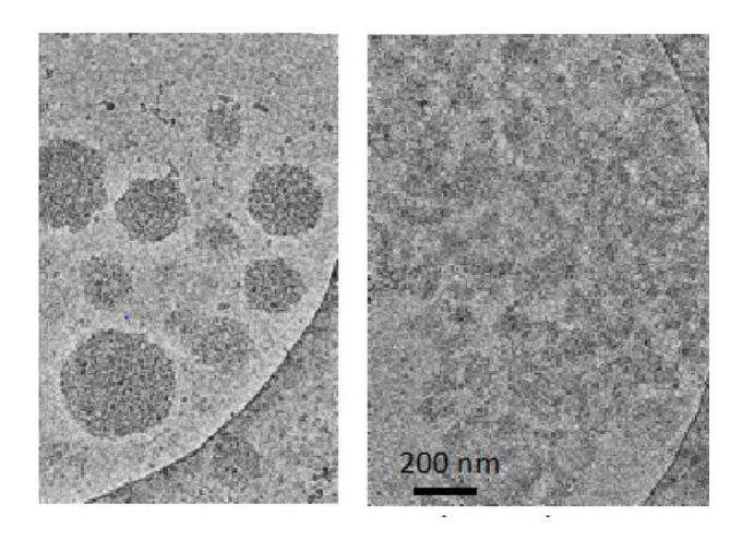
This Cryo-TEM image of native milk protein (casein) micelles in skim milk (left) and disordered open protein structures after high pressure jets at 400 megapascal (right). Notice that after processing, the casein proteins no longer aggregate as micelles. Credit: Federico Harte
