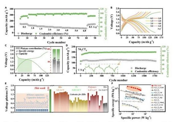
Professor Zhi Chunyi from City University of Hong Kong and his team developed battery-like electrochemical Nb<sub>2</sub>CTx MXene electrodes. This figure shows the electrochemical properties of the Nb<sub>2</sub>CTx /Zn battery. Credit: Li, Xinliang et al /DOI number: 10.1016/j.joule.2021.09.006
