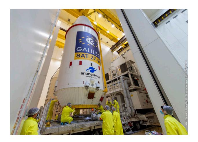
Galileo satellites 27-28 encapsulated for launch within their protective launch fairing, attached to their dispenser and atop their Fregat upper stage. This combined 'upper composite' was then placed on top of the other three stages of the waiting Soyuz launcher, ahead of their launch on Thurday 2 December at 0131 CET. Credit: ESA-CNES-Arianespace Optique Video du CSG - G Barbaste
