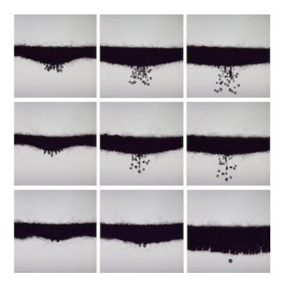
Top: Single layer dry mask shows penetration and atomization. Middle: Single layer wet mask shows reduced penetration and atomization. Bottom: Multilayer wet mask shows almost no penetration. Credit: S. Bagchi and A. Saha (UCSD).
