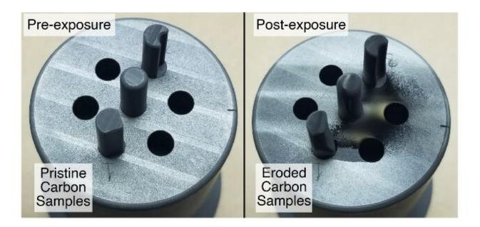
This set of carbon test samples (before, left, and after, right) was exposed to hot plasma in the DIII-D tokamak. Researchers measured the ablation behavior under this extreme heat and particle flow to simulate conditions experienced by spacecraft heat shields during atmospheric entry. Credit: UC San Diego Center for Energy Research
