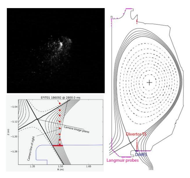
Carbon pellet spallation ("shattering") process observed in visible light (top left), full (right) and zoomed (bottom left) view of the DIII-D tokamak cross section, location of the divertor diagnostics DiMES launcher and the path of the pellet. Credit: UC San Diego Center for Energy Research.
