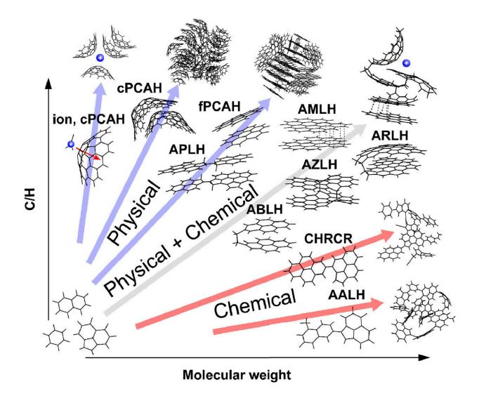
Schematic of various soot nanoparticles arranged as a function of their C/H ratio and molecular weight. Credit: Jacob Martin
