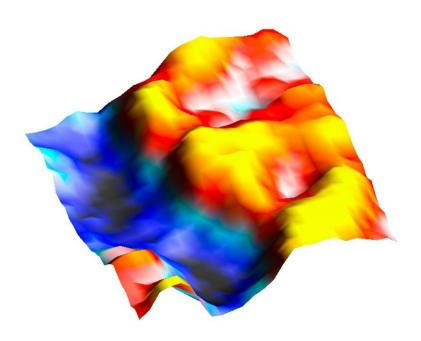
Observation of freestanding ferroelectric bubble domains by high-resolution piezoresponse force microscopy: The two blue-white spots (4 nm radius) at the right side of the image indicate bubbles. Credit: Argonne National Laboratory.)
