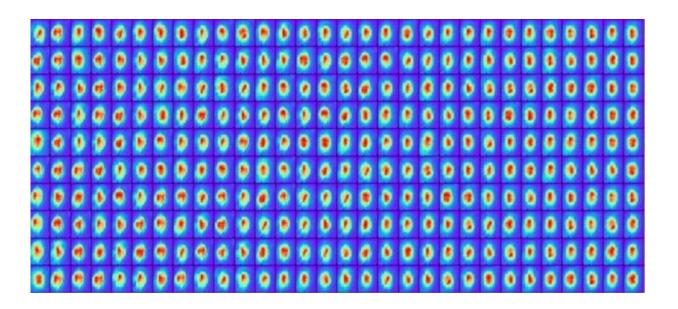
Random variations in the intensity profiles of hundreds of focused x-ray freeelectron laser pulses (shown here) reduces imaging resolution. The authors of this work combined machine learning with computational lenses to infer and reduce these variations, thus improving single-particle imaging resolution.
