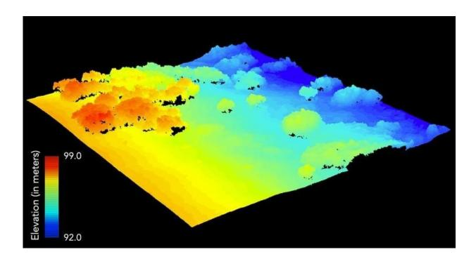
Three-dimensional rendering of surface elevation and structure of an Arctic vegetation canopy from the aerial system. Highly detailed information like this yields new insights into the distribution and structure of plants at high latitudes. Credit: Brookhaven National Laboratory
