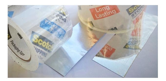
Scientists have designed a zero-carbon, zero-energy cooler that uses the most common of household items: Scotch® tape. Credit: Jyotirmoy Mandal and Aaswath P. Raman, UCLA
