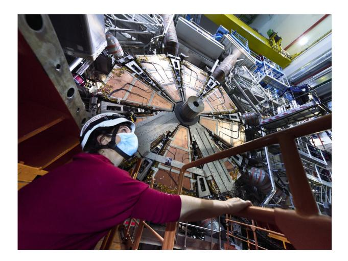
NSW "A" positioned in place inside the ATLAS experiment. Credit: CERN
