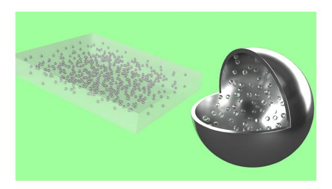
A rendering of liquid metal droplets embedded in a silicone material (left) and microscopic spheres of hollow glass enclosed in a droplet of that liquid metal (right). Credit: Scott Schrage | University Communication
