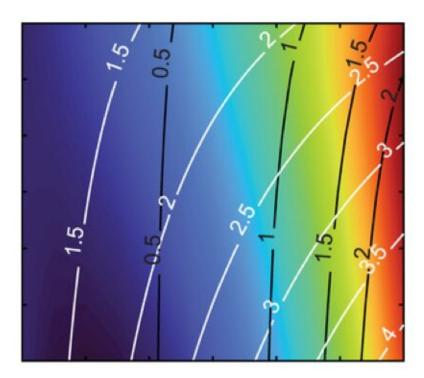
Lines indicating the proportional volumes of liquid metal and glass that will maintain a constant thermal conductivity (black) and constant density (white) in soft composite materials. Credit: Small / John Wiley & Sons
