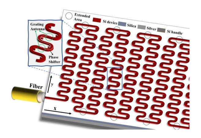
3D schematic drawing of the presented serpentine OPA design. Grating antennas, phase shifters, and the additional lengths between two serpentine sections are circled in green, white, and black, respectively. Credit: XIOPM
