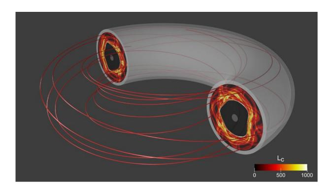
Destructive magnetic perturbations create a complex 3-D structure of magnetic field lines that randomly wander inside the tokamak. The red line shows the 3-D trajectory of an example field line, and each field line can have a significantly different trajectory. The colors of the cross-section represent the length of field line trajectory through each area, from short (black) to long (yellow) lengths. Credit: Min-Gu Yoo
