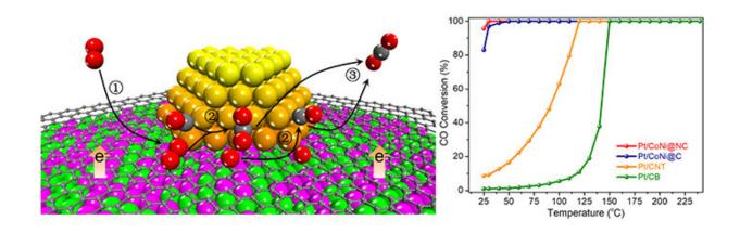
Graphene-isolated Pt from CoNi nanoparticles (PtlCoNi) for efficiently catalytic CO oxidation. Credit: HU Jingting
