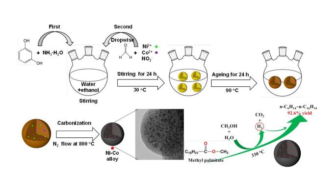
Novel carbon-coated bimetallic catalyst for in-situ aqueous phase hydrodeoxygenation. Credit: Jixiang Chen
