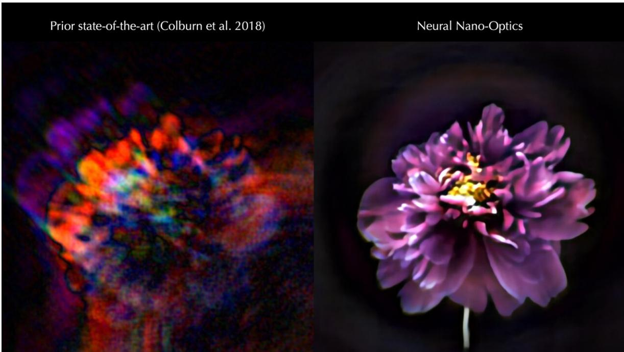
Previous micro-sized cameras (left) captured fuzzy, distorted images with limited fields of view. A new system called neural nano-optics (right) can produce crisp, full-color images on par with a conventional compound camera lens. Credit: Princeton University
