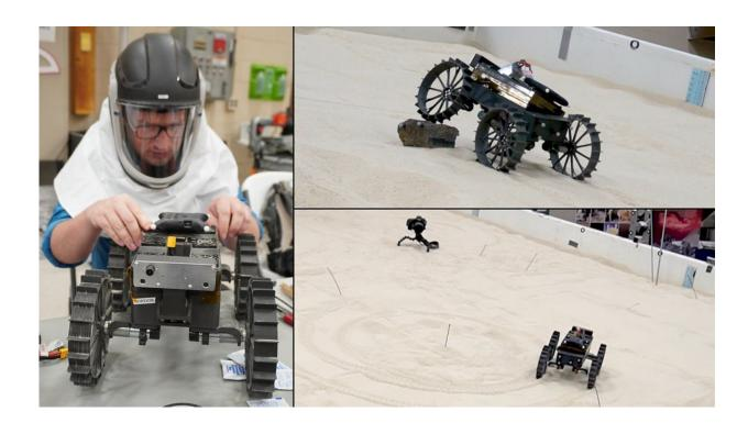
Mini-rovers designed to autonomously work together recently underwent tests at NASA's Glenn Research Center, navigating obstacles and surfaces that they could encounter on the Moon. Credit: NASA
