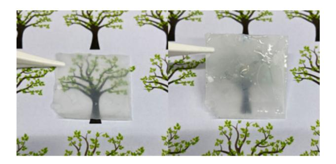
Nanocellulose-composite slides with various optical functionalities. Credit: Aalto University
