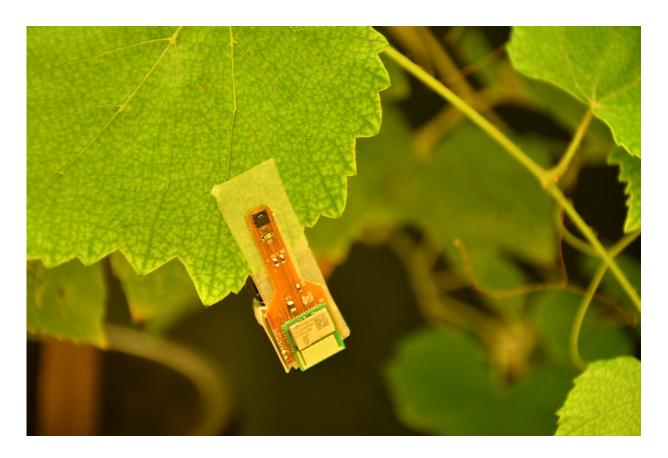
Hooks printed with the use of a photosensitive resin have been assembled together with electronics and sensors for light, temperature and humidity within a unified system, creating intelligent clips for the wireless monitoring of the plant through both sides of the leaf. Credit: IIT-Istituto Italiano di Tecnologia
