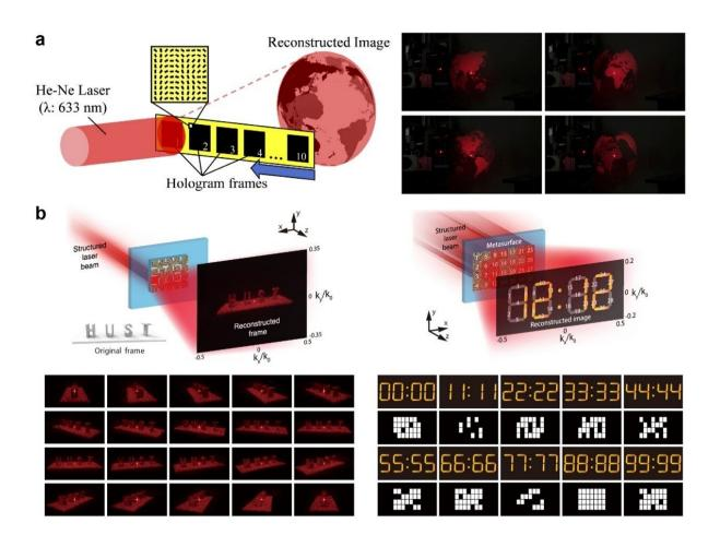
Space channel-multiplexed meta-holography. (a) Schematic of a cinematography-inspired metasurface holographic movie. Time-lapse images were reconstructed using sequentially arranged metasurface hologram frames. (b) Schematic of a space channel multiplexed metasurface. A structured laser beam opens a specific space channel in the designed sequence, and continuous frames of a holographic video are displayed. Credit: OEA
