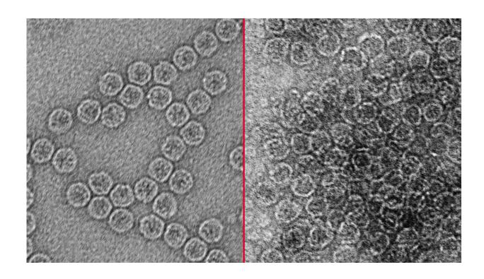
Transmission electron micrographs of a nonenveloped virus, MS2 bacteriophage, before electrocoagulation (left) and after (right). Credit: Texas A&M Engineering/Shankar Chellam and Anindito Sen
