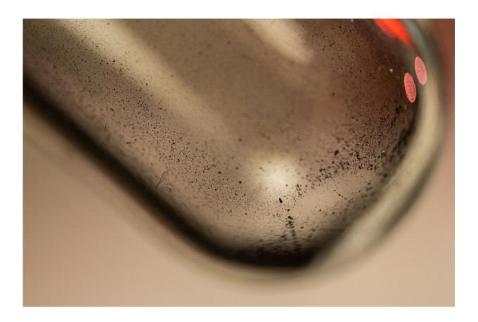
Metals settle at the bottom of a vial after being separated from other components in a crushed circuit board through flash Joule heating. The process developed at Rice University could lead to "urban mining" for valuable metals from electronic waste. Credit: Jeff Fitlow/Rice University
