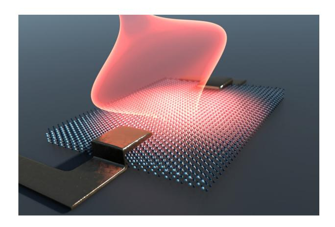
A quasi-two-dimensional crystal placed between contacts is excited by a laser pulse (red). In the irradiated region its physical properties can change dramatically on ultrashort, femtosecond time scales. This can lead to light-induced superconductivity, switching between insulating and metallic phases, or novel Floquet topological states with unusual charge transport properties. Credit: Alberto de la Torre, Dante Kennes, Martin Claassen, Simon Gerber, James McIver, Michael Sentef
