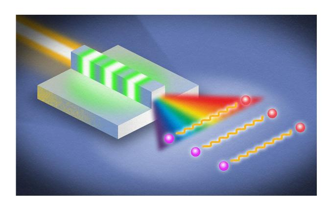
Researchers in the lab of Qiang Lin at the University of Rochester have generated record 'ultrabroadband' bandwidth of entangled photons using the thin-film nanophotonic device illustrated here. At top left, a laser beam enters a periodically poled thin-film lithium niobate waveguide (banded green and gray). Entangled photons (purple and red dots) are generated with a bandwidth exceeding 800 nanometers. Credit: Usman Javi and Michael Osadciw
