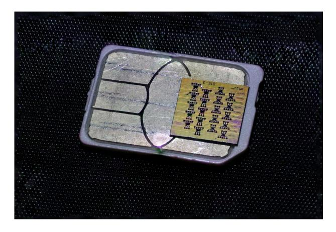
A fabricated piezoMEMS-silicon nitride chips containing multiple optical isolators. Credit: EPFL
