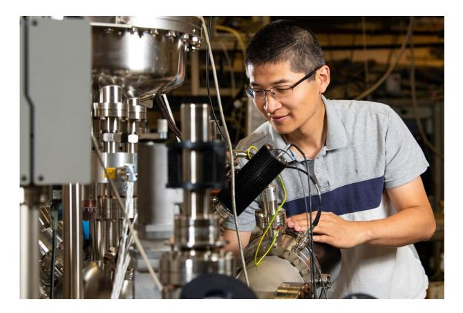
Le Wang uses an X-ray photoelectron spectroscopy instrument to measure the composition and electronic structure of synthesized thin films. Credit: Andrea Starr | Pacific Northwest National Laboratory
