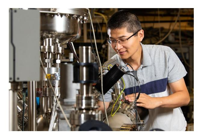
Le Wang uses an X-ray photoelectron spectroscopy instrument to measure the composition and electronic structure of synthesized thin films. Credit: Andrea Starr | Pacific Northwest National Laboratory
